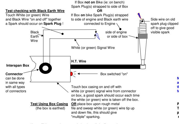
Note: This operation can only be done if the Battery is charged on box, or you have a "remote" charging/signal lead loom whereas you can put box "on charge" at the same time as doing this test.
